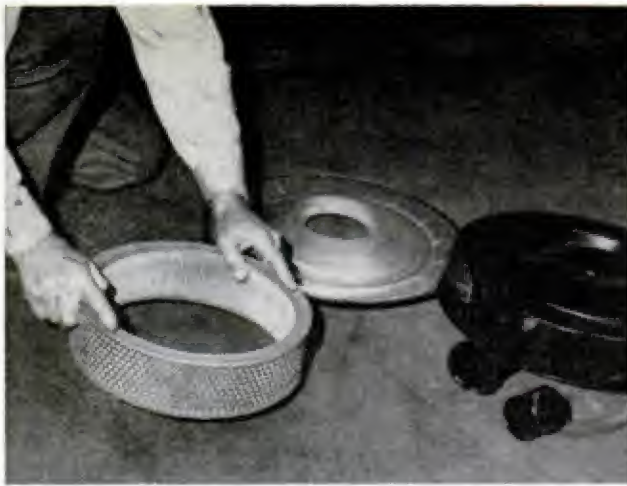
AIR CLEANER is removed from its housing on top of carburetor. New air cleaner is installed in seconds
